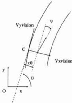
Figure 2: Parameters given by the vision algorithm in their reference
