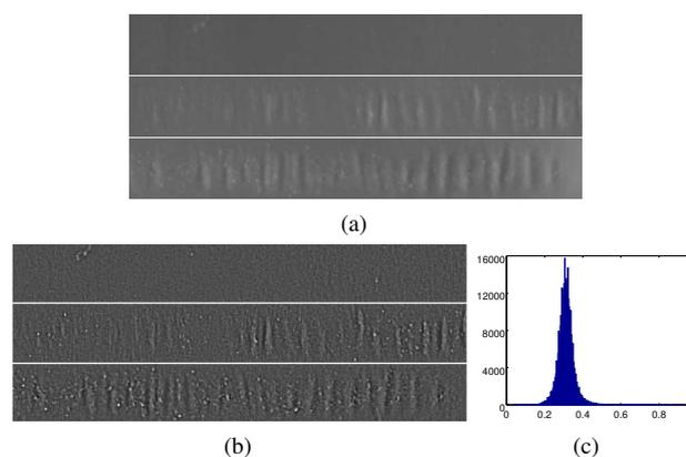
Figure 1: (a) IGT sample (coated board); (b) after preprocessing. Images (a) and (b) are divided into 3 pieces from top to bottom for better presentation; (c) gray-level histogram of preprocessed sample.
