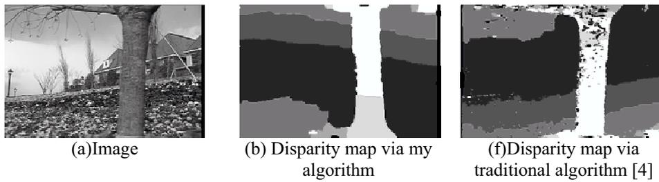
Figure 5. The examples of disparity estimation results.
