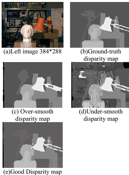
Figure2. Disparity maps via different smooth energy coefficients.
