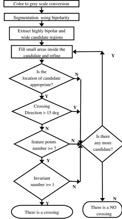
Figure 1: Flow diagram of the proposed method.
