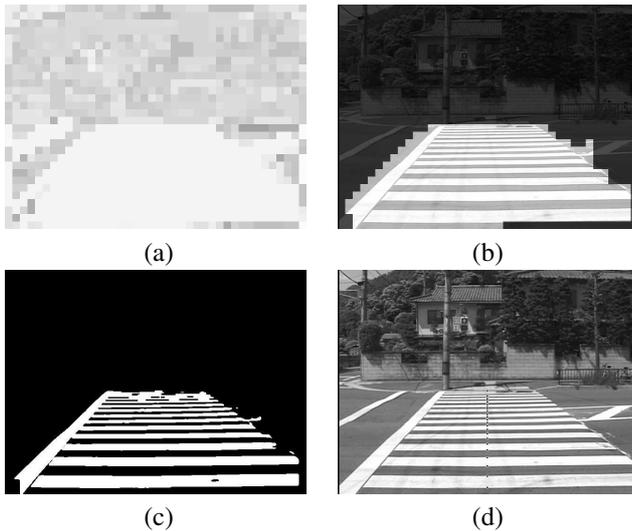
Figure 3: Different steps in detecting the existence of a crossing for the image of Fig. 2(a): (a) bipolarity of each segmented region, (b) candidate crossing area, (c) binarized crossing area (d) extracted feature points marked on the image.
