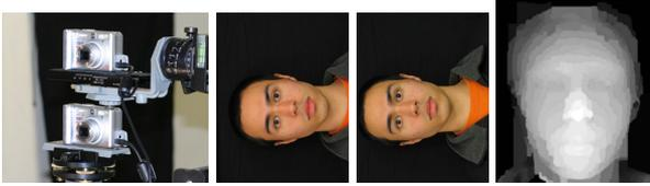
**Figure 1. The From left to right: The camera setup, the resulting image pair in vertical epipolar position and the depth map obtained using KZ1.**
