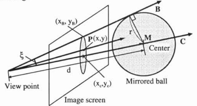
Figure 3. Calculation of the spatial position of the ball
