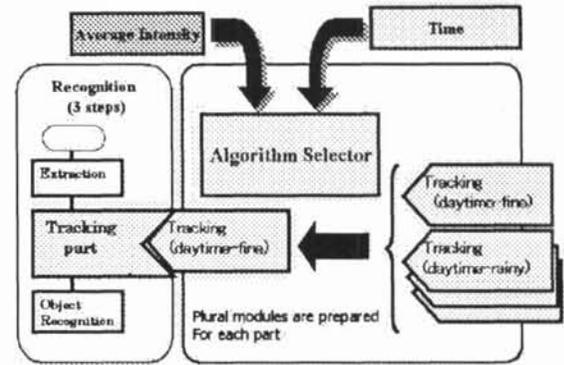
Figure 4: Dynamic Algorithm Selection in Moving Object Recognition Part
