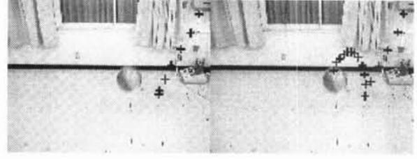
Figure 4: The results of a single state CONDENSATION algorithm(left) and the mixed-state CONDENSATION algorithm(right): left figure shows the tracker didn't track after bounce state, while in the right figure it tracks after bounce state successfully.
