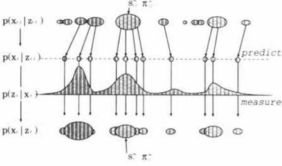
Figure 3: Probability transition at one timestep in the CONDENSATION algorithm.
