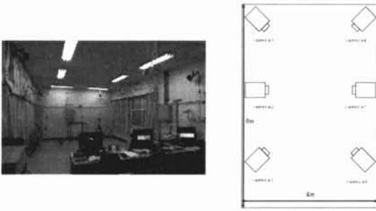
Figure 6: The camera positions: six cameras are set up in this room whose size is  $8m \times 4m \times 3m$
