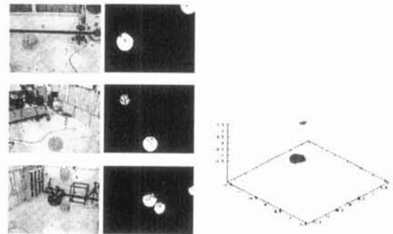
Figure 2: Background subtraction and 3D-shape from silhouettes of balls. Left: 3 view images including moving balls. Middle: Background subtraction images. Right: Reconstructed 3D positions of balls.
