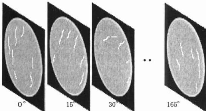
Fig. 2-3: A volume of correlation coefficient images Sorted in the order of the kernel orientation. They are processed as if the both ends were connected each other.
