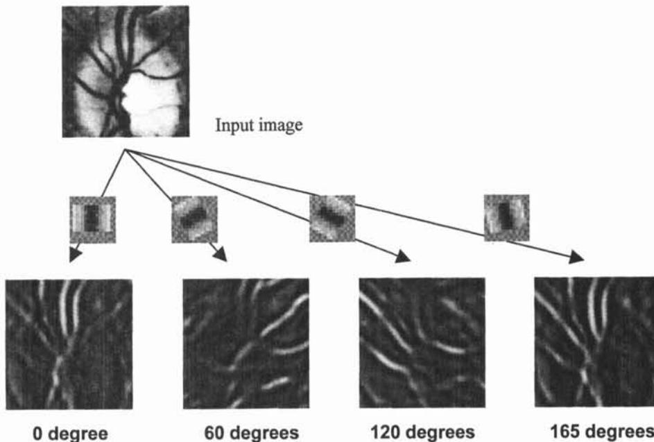
Fig. 2-2: Creation of twelve correlation coefficient images. The original range of correlation coefficient is [-1,1]. The range was converted to [0.255] in order to make grayscale images.
