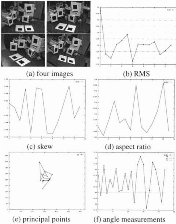
Figure 1: (a) Four from 14 images. Image size is  $640 \times 480$ . (b) RMS errors for each view after projective bundle adjustment (24 point matches). (c) skew (d) aspect ratio (e) principal points (f) angle measurements of the orthogonal angles. The true angles are 90 degrees.
