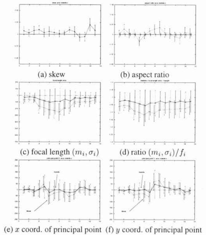
Figure 2: Statistics of simulation results after 100 runs when input noise level is 0.5pixel for each of the image coordinates. Bold lines (—) are for bundle adjustment and dashed lines (- - -) for the linear algorithm. Vertical line segments denote one standard deviation ranges from the mean values.
