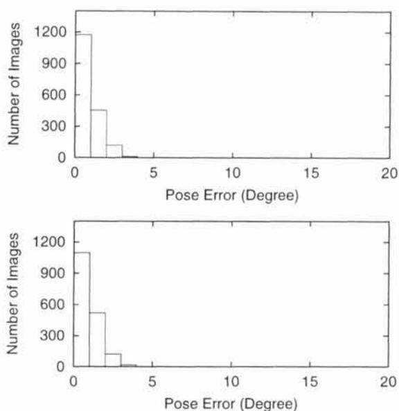
Figure 4: Pose estimation error for noisy images. Added noise is 5% (upper) and 10% (lower).
