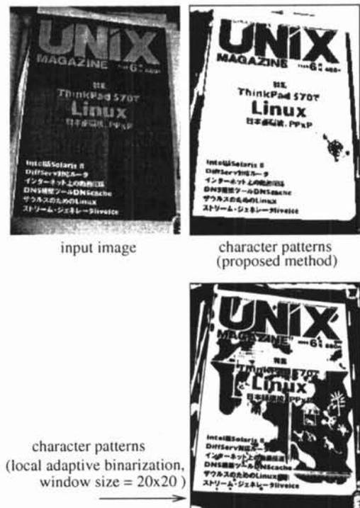
Figure 6: Character pattern extraction from the image with complex backgrounds (UNIX MAGAZINE, June, 2000, ASCII CORP.)
