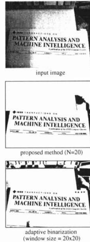
Figure 5: Character pattern extraction from the image with simple background (IEEE Trans. PAMI, Vol.22, No.3, 2000.)
