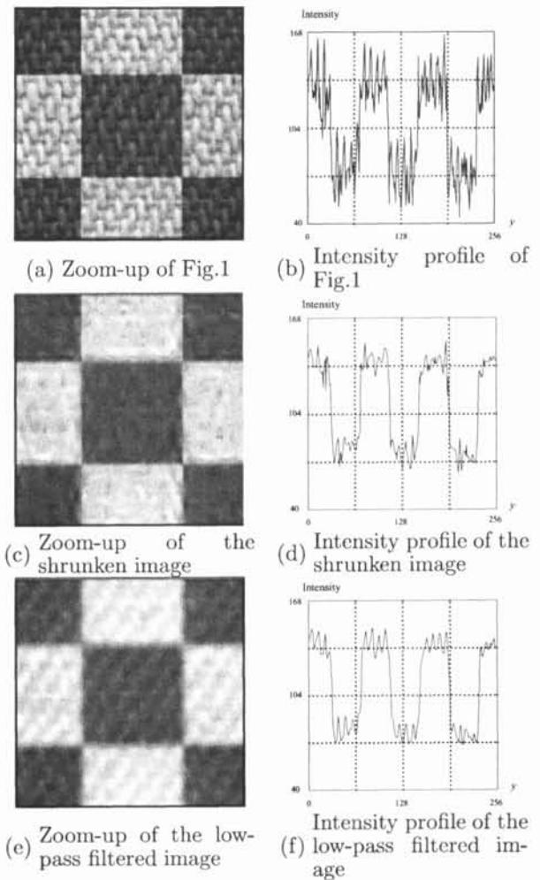
Figure 2: The results of removing the intensity variations caused by textures
