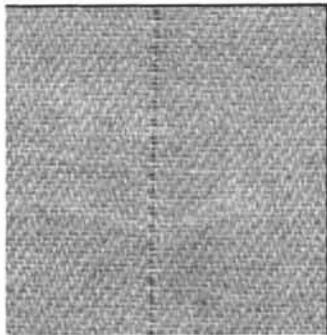
Figure 3: A textile surface containing defects
