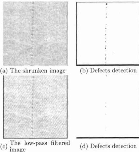
Figure 4: The result of defects detection of Fig.3
