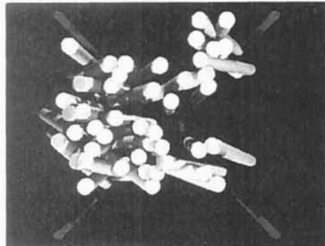
Fig. 12 The image reconstructed from the measured fiber orientation
