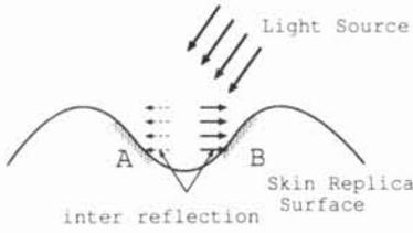
Figure 3: Mechanism of the inter reflection on skin replica surface.
