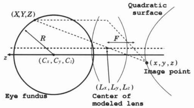
Fig. 4: Coordinate system and parameters for the modeled optical system of the eye lens with the contact enlarging lens
