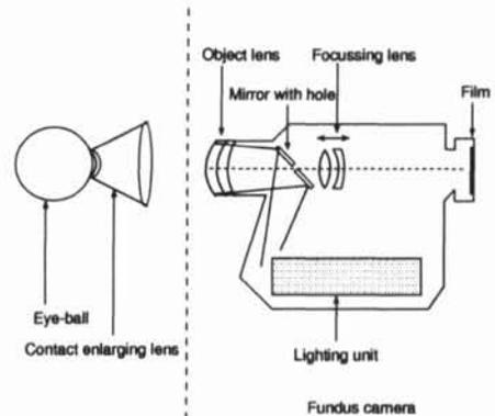
Fig. 1: Optical system of fundus camera and human eye
