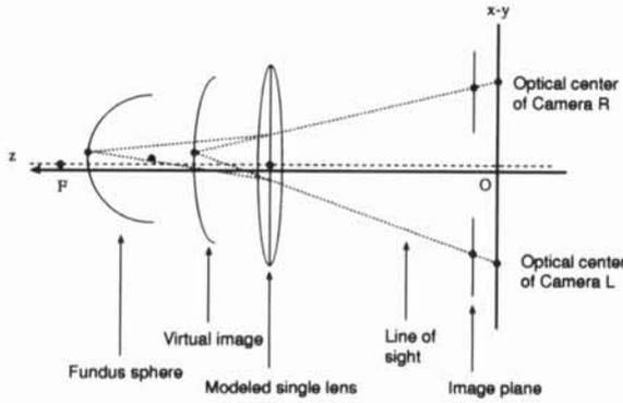
Fig. 2: Optical model for stereo fundus images (without contact enlarging lens)
