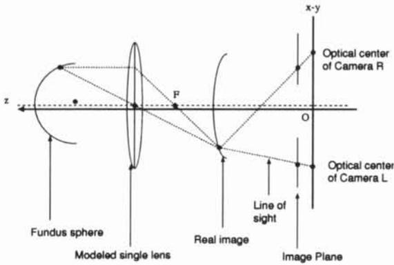
Fig. 3: Optical model for stereo fundus images (with contact enlarging lens)
