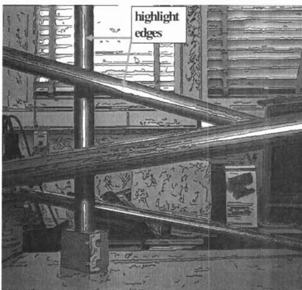
Figure 2 : Canny gradient image : virtual edges created by highlights.
