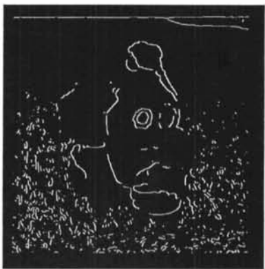
Figure 19: Edge intensity image by the first derivative of a Gaussian with \sigma=2 , ( Tr=50 )
