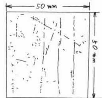
Fig.7 The result of logical EXOR operation for flaw-and-defect identification.
