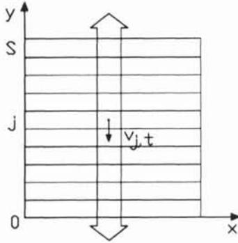
Figure 3: Optical flow field segments in the image plane at time  $t$ .
