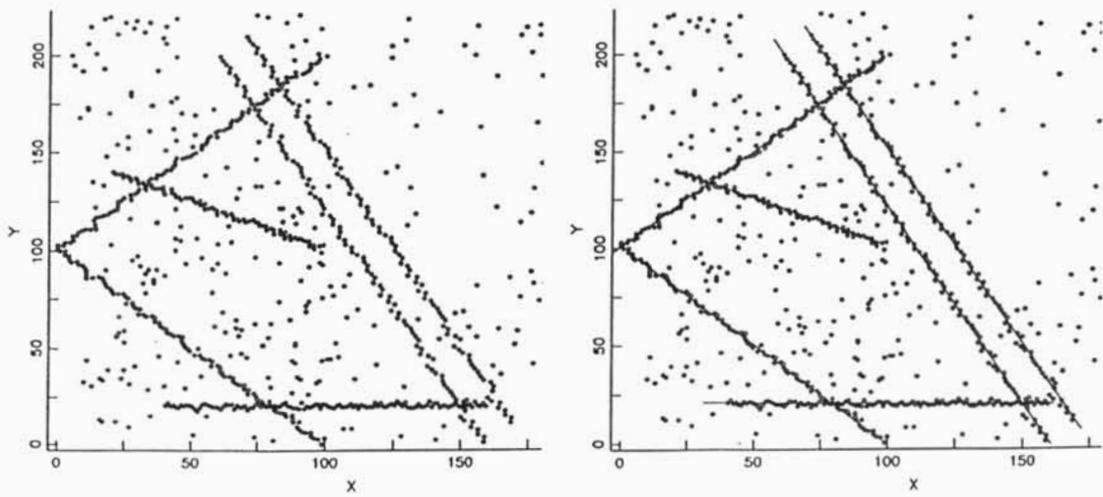
Figure 2: Multiple line segment detection example. The input data is on the left. The data with computed line segments overlaid is on the right.
