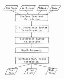
Figure 4. O.P. Views Generation Flow Diagram.
