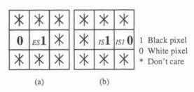
Fig.2 Necessary conditions for external start point(ES) and internal start point(IS)
