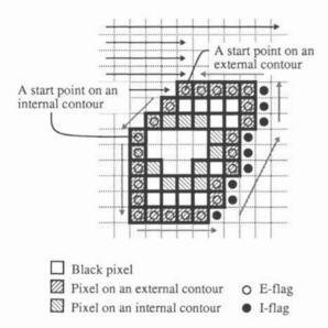
Fig.1 Start point detection and external contour tracking
