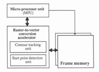
Fig.3 Block diagram of fast raster-to-vector conversion system
