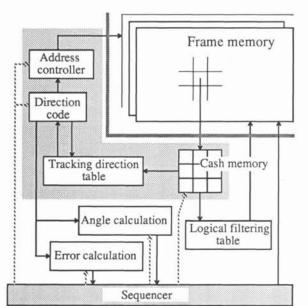
Fig. 5 Configuration of contour tracking unit
