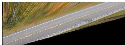
Figure 4. Affine rectification recovers the original lanes in Fig. 1.
