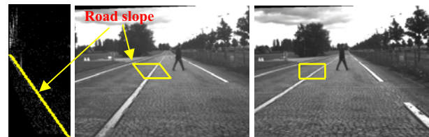
Figure 4. Principle of a sheared correlation window adapted to the road surface.
