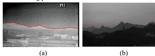
Figure 1 (a) Horizon and (b) peaks from IR images[1]
