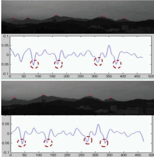
Figure 3 Curvature value due to the different frame
