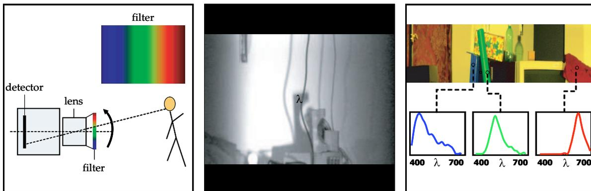
(c) Multispectral imaging using generalized mosaicing.
