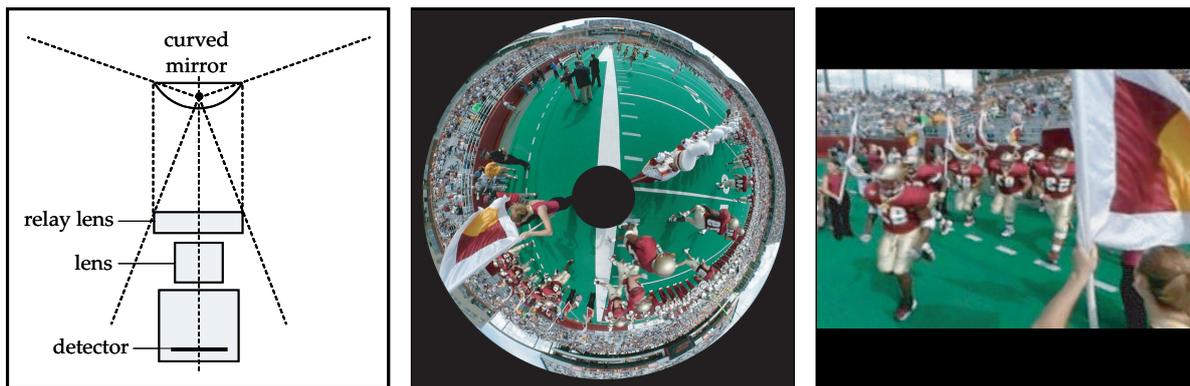
(a) Wide-angle imaging using a catadioptric camera.
