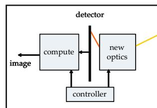
Figure 3. A programmable imaging system is a computational camera whose optics and software can be varied to emulate different imaging functionalities.
