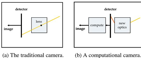
Figure 1. (a) The traditional camera is based on the principle of the camera obscura and produces a linear perspective image. (b) A computational camera uses novel optics to capture a coded image and a computational module to decode the captured image to produce new types of visual information.
