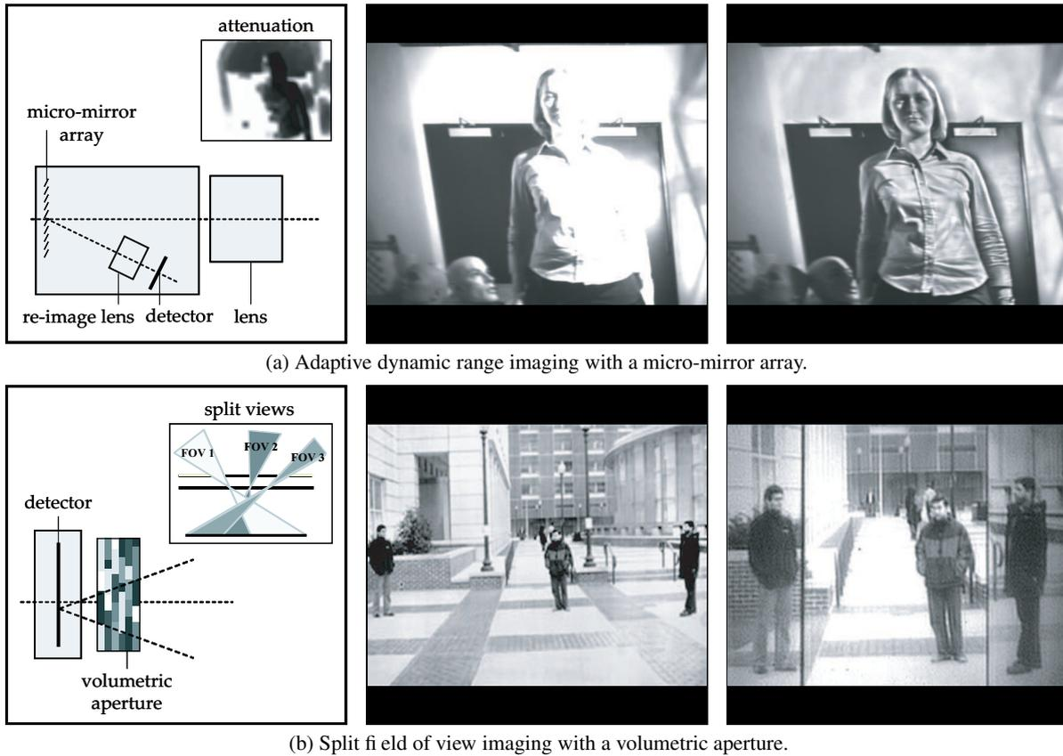
(a) Adaptive dynamic range imaging with a micro-mirror array.
