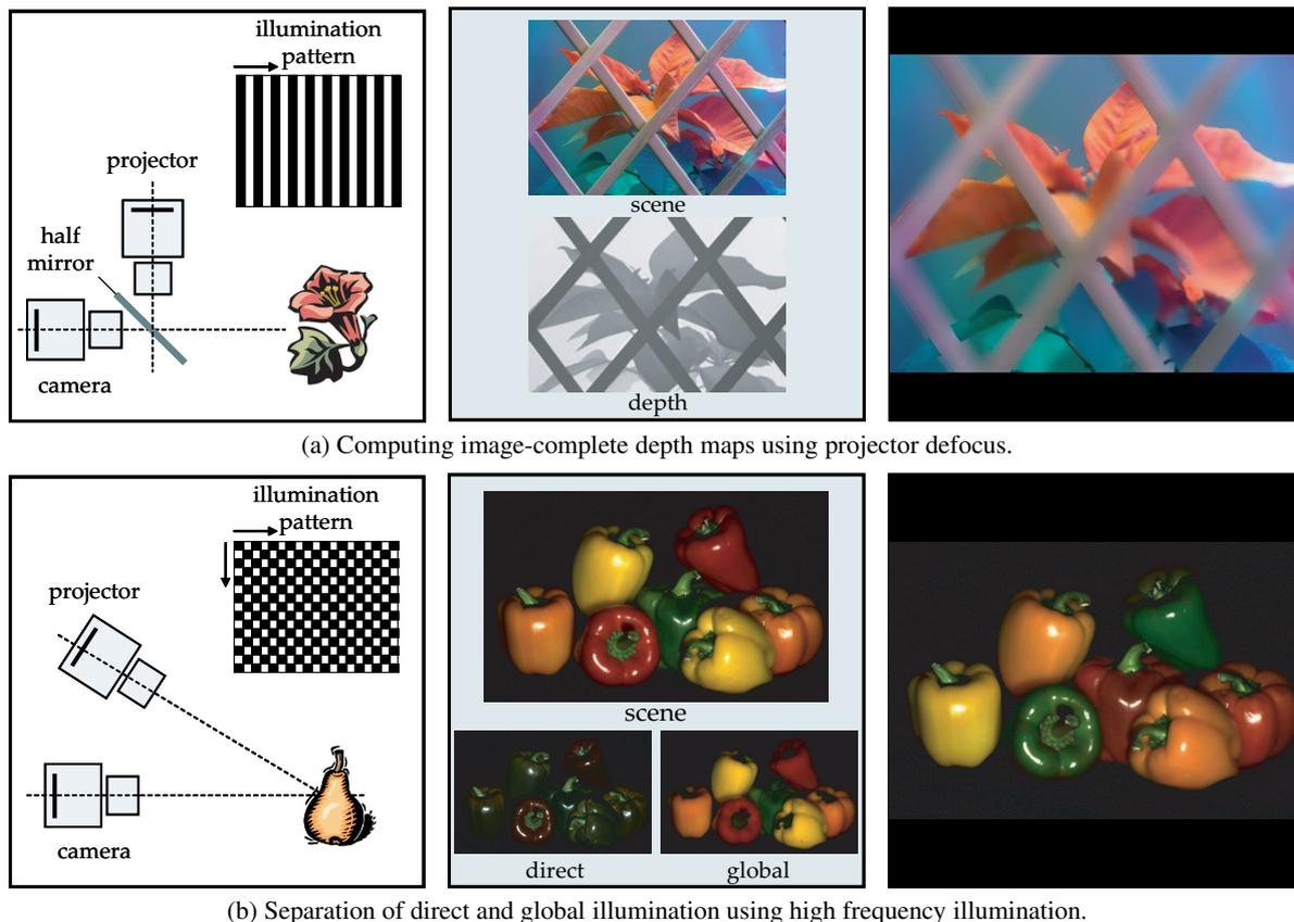
(a) Computing image-complete depth maps using projector defocus.
