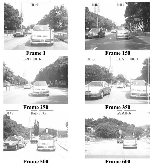
Figure 5. A sequence of vehicle tracking images with distance information
