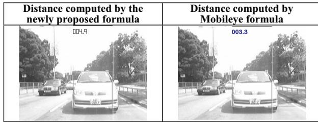
Figure 4. The camera-to-vehicle distance computed by the newly proposed formula
