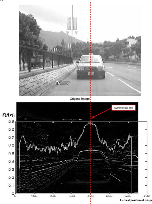
Figure 1. Symmetrical measurement using gradient image with horizontal edges as input
