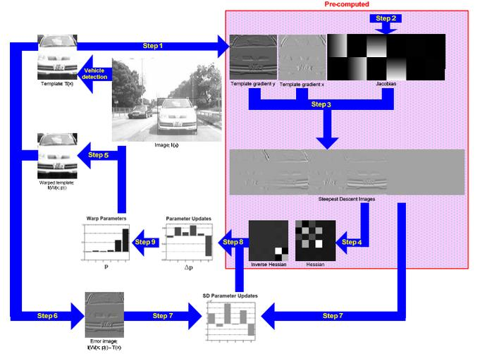
Figure 3. The framework of the inverse compositional algorithm
