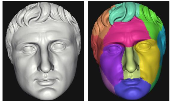
Fig. 6. The result of distinguishing region detection. (a): an input model; (b): detected feature regions. Number of clusters is set to 12 in this example.
