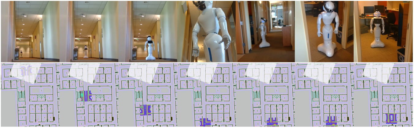
Fig. 9. Navigation with our system using external SLAM device. Lower sequence is floor map in GUI. First, Pepper walks long corridor and then turn at the corner. Finally, Pepper enters a room and reaches to the destination.
