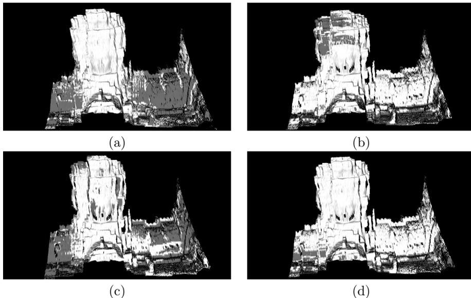
Figure 9: Case1: Comparisons with the range data obtained by the ground-based sensor. The white regions indicate where the distances of the corresponding pairs are less than 1.0 cm. (a)The original distorted range data by FLRS. (b)The range data rectified by the hardware-based method. (c)The range rectified by the 3DA-based method. (d)The range data rectified by the SFM-based method.
