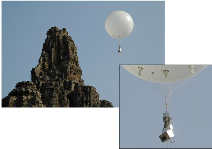
Figure 3: The Flying Laser Range Sensor
