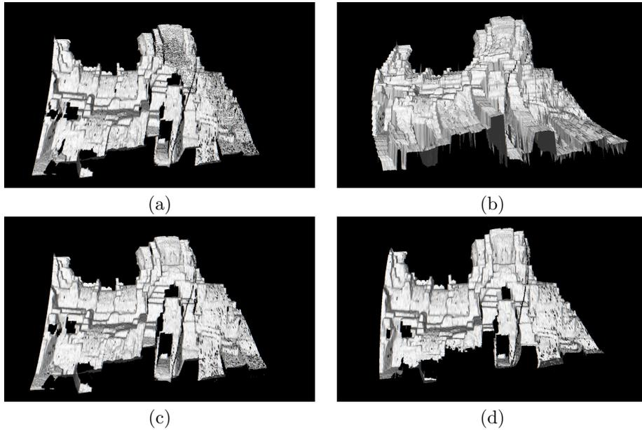
Figure 12: Case2: (a)The original distorted range data by FLRS. (b)The range data rectified by the hardware-based method. (c)The range data rectified by the 3DA-based method. (d)The range data rectified by the SFM-based method.
