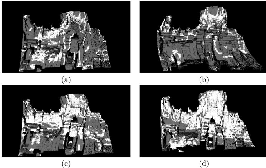
Figure 13: Case2: Comparisons with the range data obtained by the ground-based sensor. The white regions indicate where the distances of the corresponding pairs are less than 1.0 cm. (a)The original distorted range data by FLRS. (b)The range data rectified by the hardware-based method. (c)The range data rectified by the 3DA-based method. (d)The range data rectified by the SFM-based method.
