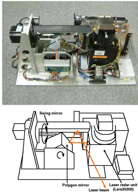
Figure 6: Interior of a scanner unit (25m sensor)
