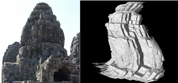
Figure 4: A sample snapshot compared with the distorted range data obtained by the FLRS
