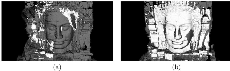
Figure 17: Case3: Comparisons with the range data obtained by the ground-based sensor. The white regions indicate where the distances of the corresponding pairs are less than 1.0 cm. (a)The original distorted range data by FLRS. (b)The range data rectified by the SFM-based method.
