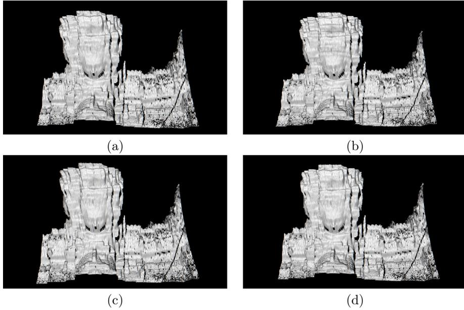
Figure 8: Case1: (a)The original distorted range data by FLRS. (b)The range data rectified by the hardware-based method. (c)The range data rectified by the 3DA-based method. (d)The range data rectified by the SFM-based method.
