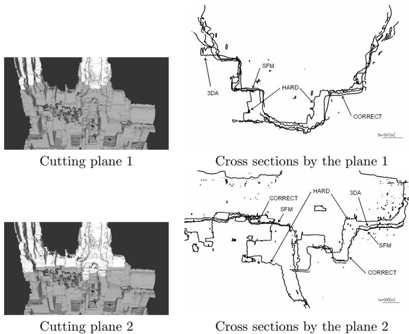
Figure 14: Case2: Cross sections of four models; "CORRECT":the correct model by Cyrax2500. "HARD": the range data rectified by the hardware-based method. "3DA": the range data rectified by the 3DA-based method. "SFM": the range data rectified by the SFM-base method.
