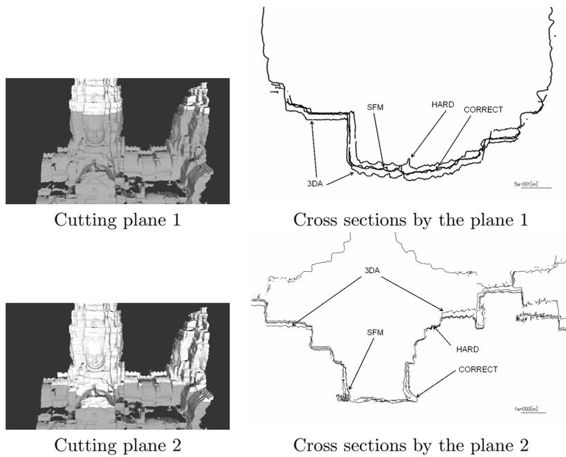
Figure 10: Case1: Cross sections of four models; "CORRECT":the correct model by Cyrax2500. "HARD": the range data rectified by the hardware-based method. "3DA": the range data rectified by the 3DA-based method. "SFM": the range data rectified by SFM-based method.
