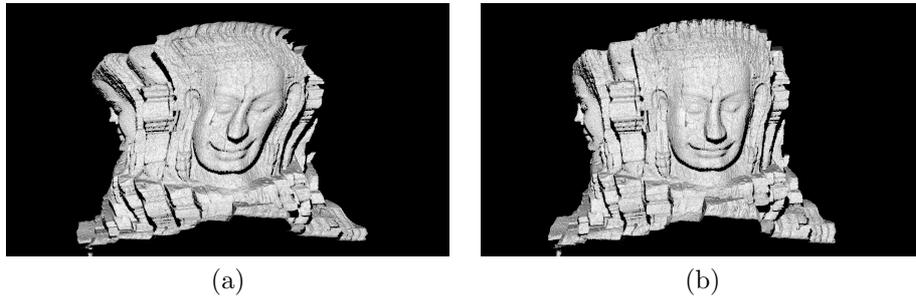
Figure 16: Case3: (a)The original distorted range data by FLRS. (b)The range data rectified by the SFM-based method.
